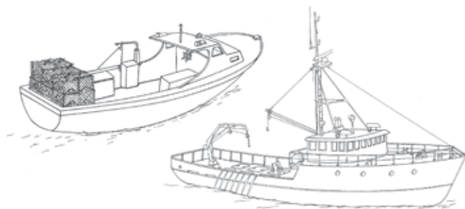
Illustration of a small trap setter (top) and a large trap setter (bottom)
