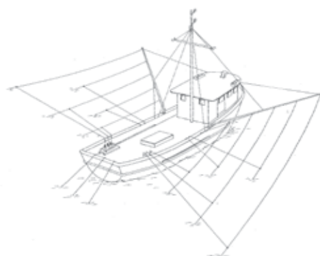
Illustration of a troller with multiple lines deployed from the outriggers (poles to the side) and stern
