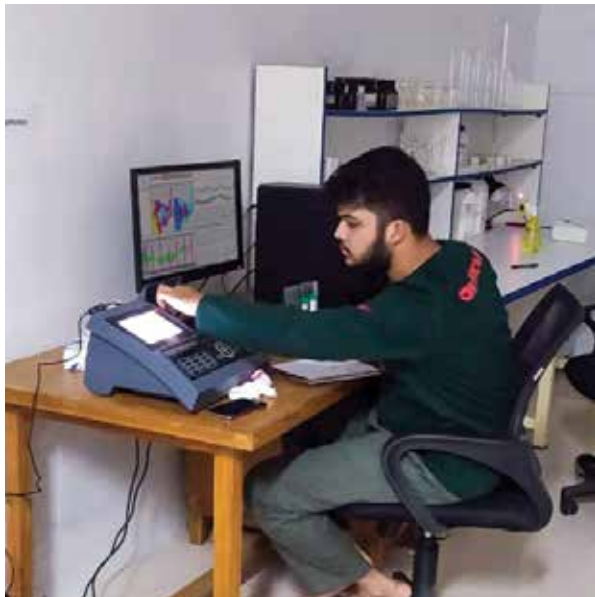
A BMU student is using spectrophotometer to measure the concentration of a compound in an aqueous solution
