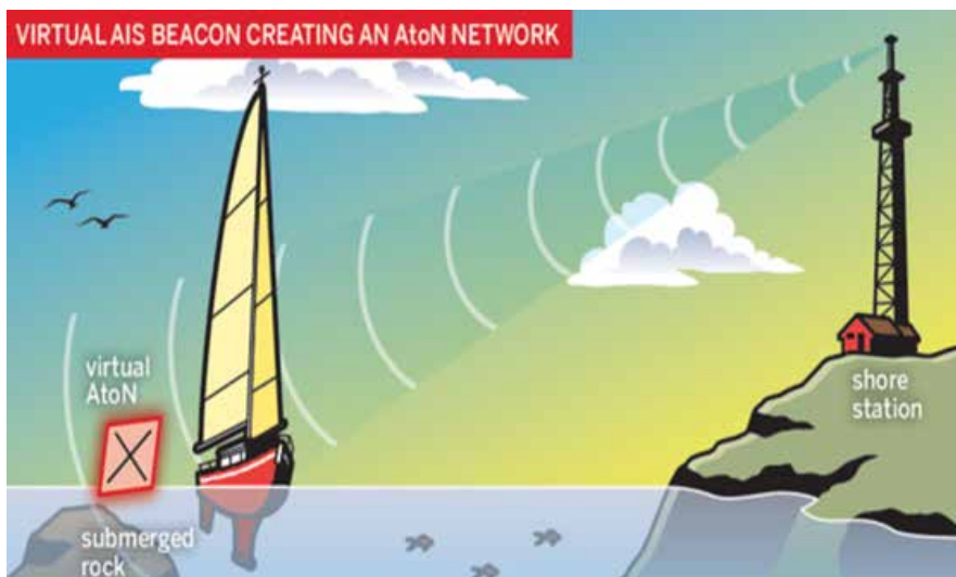
Picture no. 3. A shore station transmitting AIS signal and a sailing vessel will find a virtual AtoNon RADAR/ECDIS/AIS receiver and avoid a submerged rock very efficiently. (Source: Peter Nielsen, www.sailmagazine.com , June 12, 2012)
