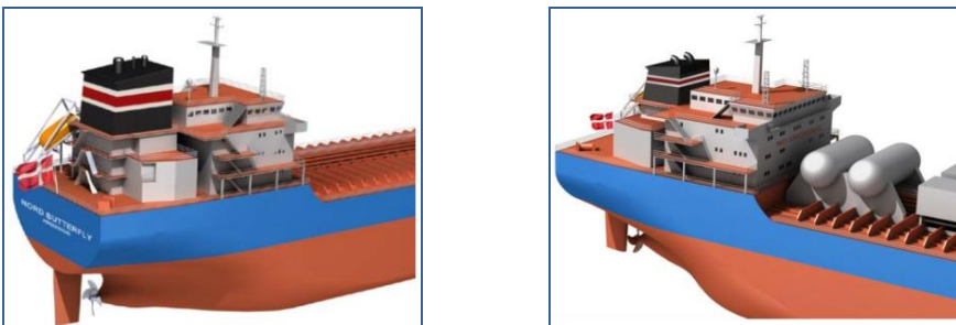
Figure 6: Aft Ship with Scrubber installed having enlarged funnel and LNG tank on main deck
